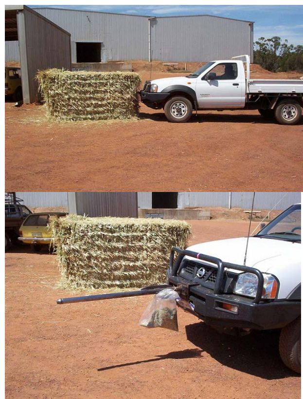
Figure 4. (top) Driving corer into hay bale and (bottom) corer with hay sample in bag. Courtesy of Leo den Hollander.
